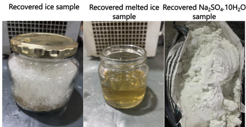
Figure 3 Samples of the recovered ice, melted ice and  $\text{Na}_2\text{SO}_4 \cdot 10\text{H}_2\text{O}$  (60%).
