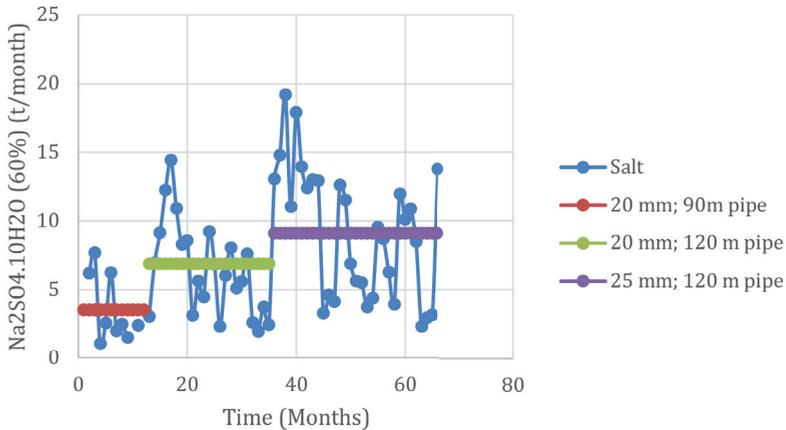
Figure 1 Salt recovery with cooling over time (from More et al. 2025).
