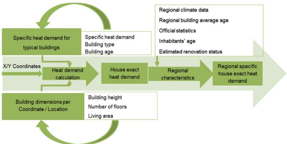
Figure 1 Algorithm to predict address-specific heating demands based on geospatial and statistical data
