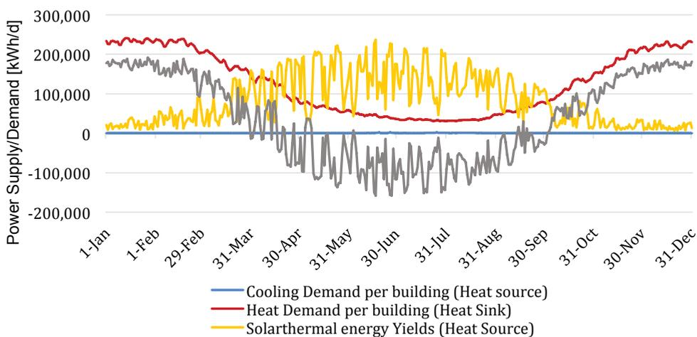
Figure 3 Seasonal progression of cooling requirements, heating requirements, solar thermal yields and the resulting heat withdrawals / injections
