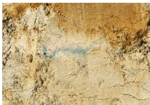
Figure 2 Blue staining found on the tailings dam in Welkom, South Africa. This is believed to be an Fe-CN compound and is ~3 cm in length.
