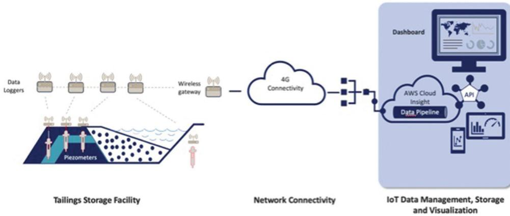
Figure 12 High level monitoring solution architecture
