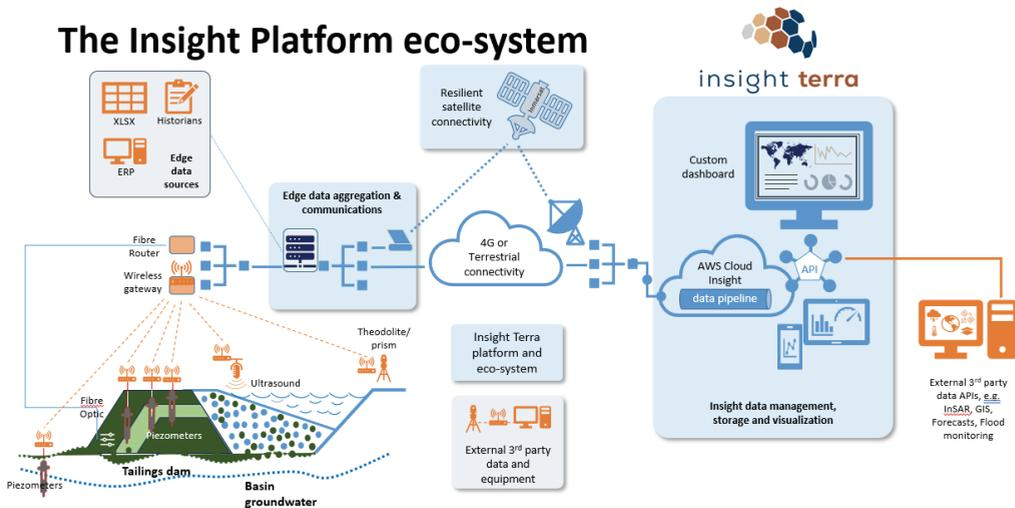
Figure 3 A monitoring system eco-system
