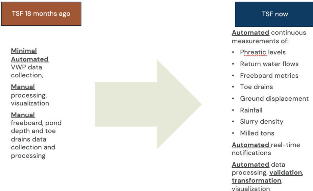
Figure 13 High level monitoring solution architecture
