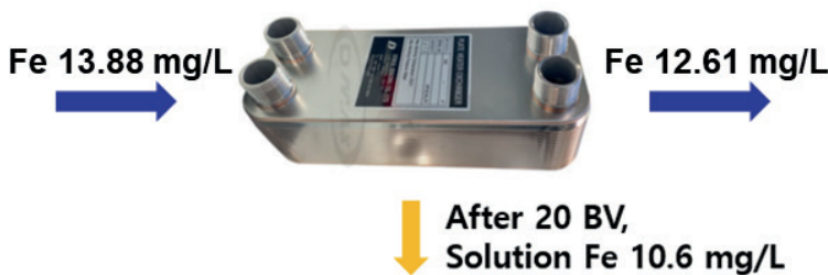
Figure 3 Results of continuous flow experiments and washing assessment of heat exchangers using mine water at Dongwon coal mine
