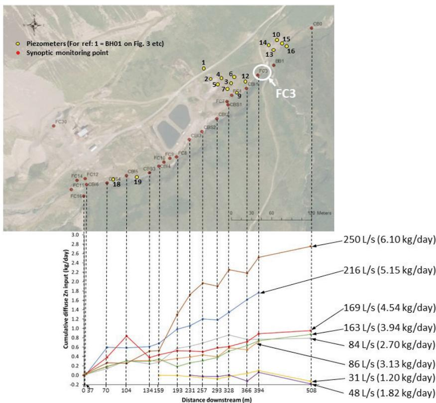
Figure 2 Cumulative diffuse filtered zinc input to the Coledale Beck during reach-scale synoptic mass balance monitoring. Flows are shown for monitoring point FC3 with zinc load at FC3 in brackets (High resolution (25cm) vertical aerial imagery, EDINA Aerial Digimap Service, <https://digimap.edina.ac.uk>)
