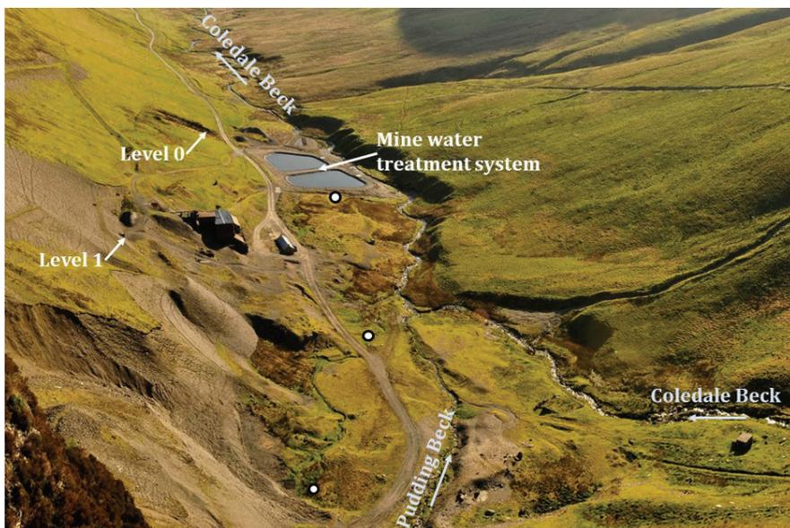
**Figure 1** Force Crag mine and Coledale Beck, showing locations of abandoned mine buildings, mine adits (levels), groundwater upwellings of metal-contaminated water (white circles), and mine water treatment system (Photo reproduced with permission of John Malley)
