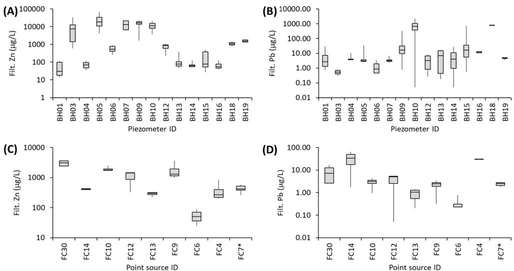
**Figure 3** Box plots of filtered (Filt.) Zn and Pb concentrations at various locations in the Force Crag mine catchment, showing (A) Zn concentrations in groundwaters, (B) Pb concentrations in groundwaters, (C) Zn concentrations of point sources and (D) Pb concentrations of point sources (See Figure 2 for locations; note: BH02 dry on all occasions).
