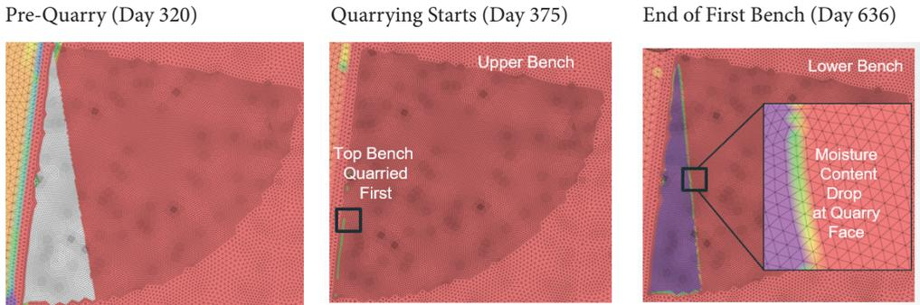
Figure 5 Simulation Results Showing Moisture Content in Walls
