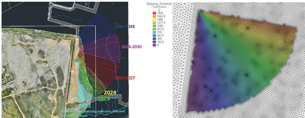
Figure 3 Example of Mine Sequencing in Feflow using User Defined Equations to form Nodal Distributions
