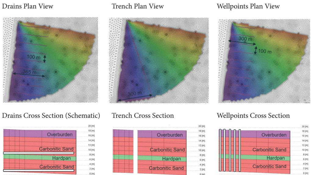
Figure 6 Model Representation of some of the Dewatering Approaches
