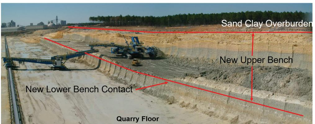
Figure 2 Quarry showing Benches and Bucket Wheel Excavator (Holcim US Inc ,2008)
