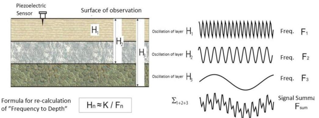
Figure 2 MSR Measurement and Data Collection Illustration
