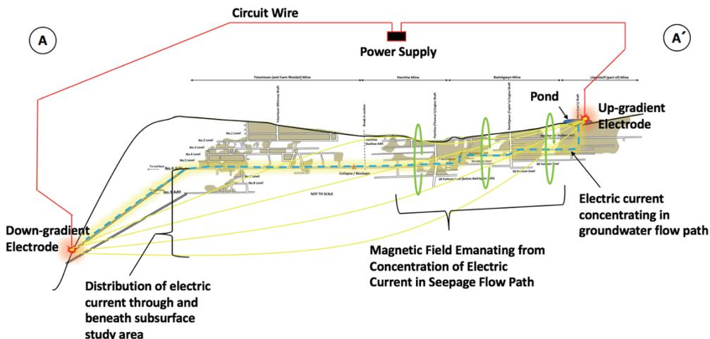
Figure 3 Cross-sectional Schematic of Willowstick Technique at Abandoned Mine
