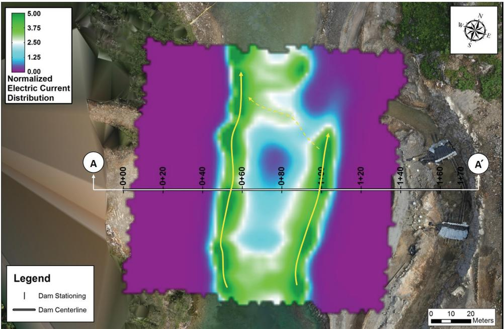
Figure 7 Willowstick Method Results (Plan View)
