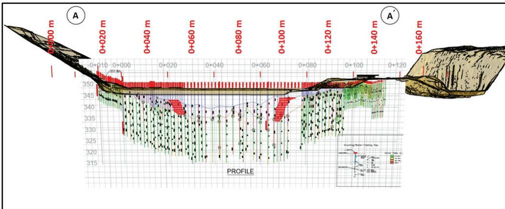
Figure 6 Longitudinal Profile As-built Drawing of Grout Curtain
