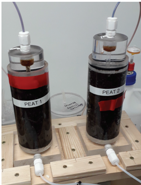
Figure 2 Peat column experiment set-up (Geochem Ltd).
