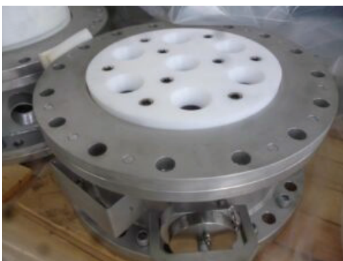
Figure 1 Aachen reactor cartridge that introduces gas under pressure to generate fine gas bubbles
