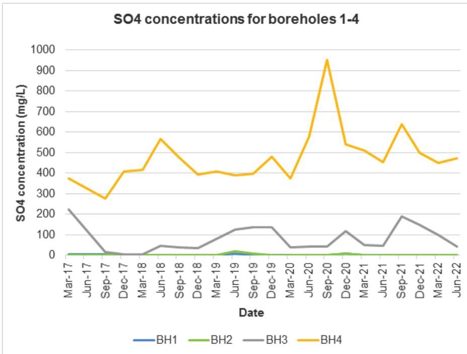
Figure 2 Borehole sulfate concentrations since the commencement of irrigation. BH1 – deep upstream, BH2 – shallow upstream, BH3 – deep downstream, BH4 – shallow downstream
