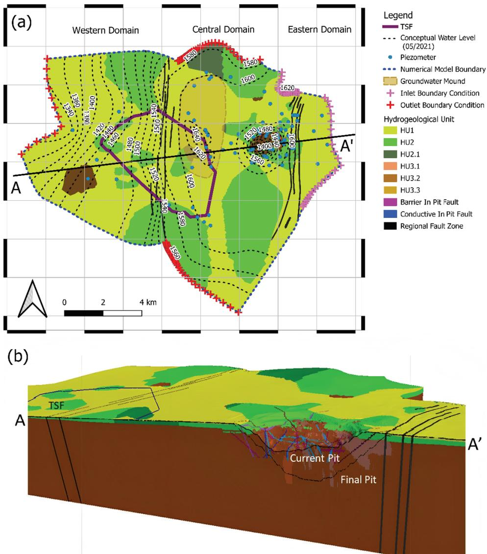
Figure 1 Conceptual and numerical groundwater model. (a) Plan view; (b) Numerical model isometric view
