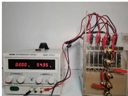
Figure 1 Electrocoagulation reactor scheme (batch)
