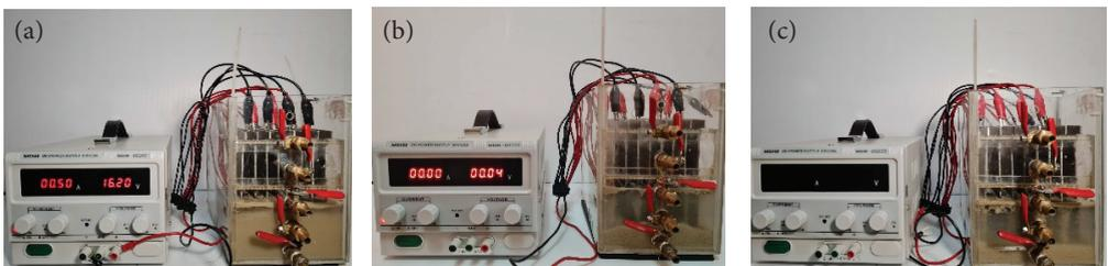
Figure 3 (a) Electrocoagulation on 15<sup>th</sup> minute with 0.5 A current (b) electrocoagulation on 45<sup>th</sup> minute with 2 A current, dan (c) after settling for 60 minutes ( $t_{ec} = 15$  minutes,  $I = 0.5$  A)
