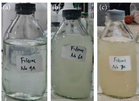
Figure 6 Electrocoagulation supernatant on (a)  $I = 2\text{ A}$ ,  $t_d = 15\text{ minutes}$ , (b)  $I = 2\text{ A}$ ,  $t_d = 45\text{ minutes}$ , and (c)  $I = 0,5\text{ A}$ ,  $t_d = 15\text{ minutes}$
