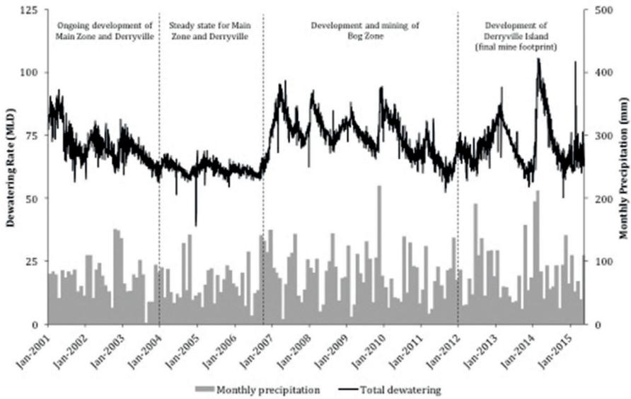
Figure 2 Dewatering rates from 2001 to 2015.
