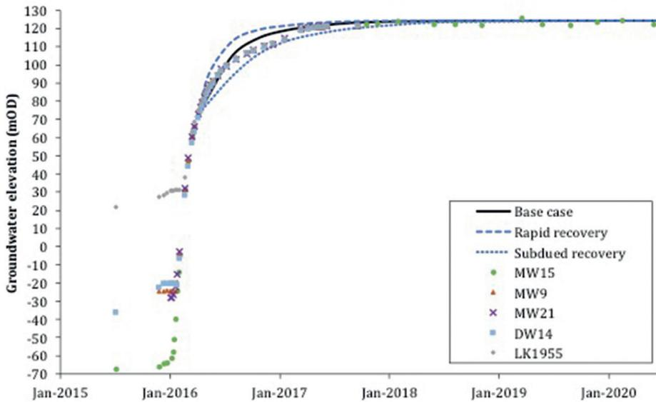
Figure 3 Groundwater recovery predictions and monitoring data.
