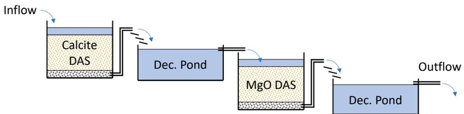
Figure 1 Schematic setup of the calcite-DAS + MgO-DAS reactors of the field trial at Cwm Rheidol.
