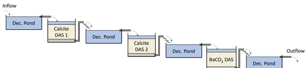
Figure 2 Schematic setup of the calcite-DAS + BaCO<sub>3</sub>-DAS laboratory columns for Parys Mountain.
