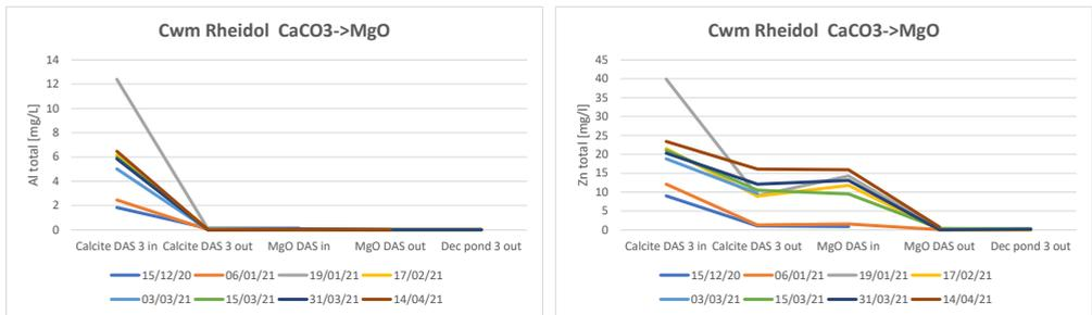
Figure 4 Evolution of total Al (left) and Zn concentrations (right) along the Cwm Rheidol treatment train.
