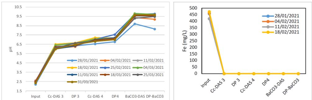
Figure 5 Evolution of pH (left) and total iron concentrations (right) along the Parys Mountain laboratory columns.
