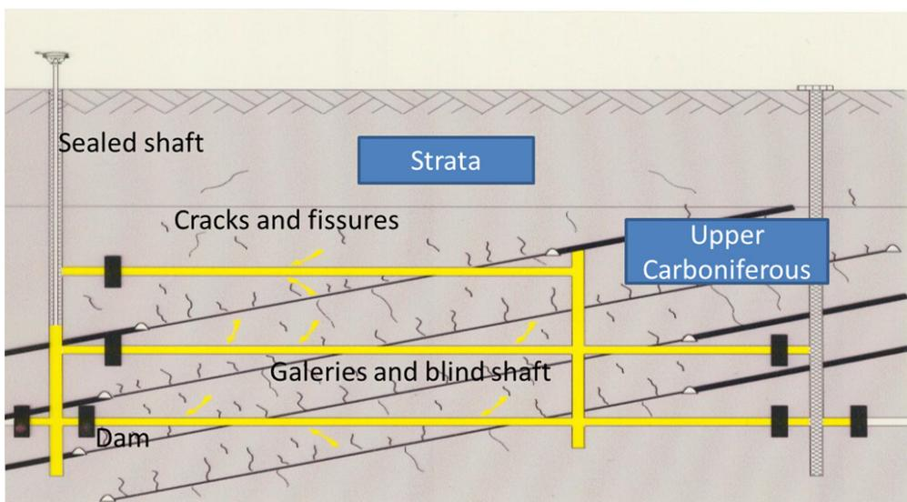
Figure 1 Schematic methane pathways to the surface (FZN).
