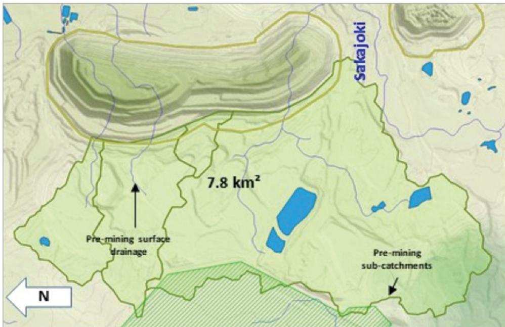
Figure 2 Pre-mining drainage system near the Main pit.
