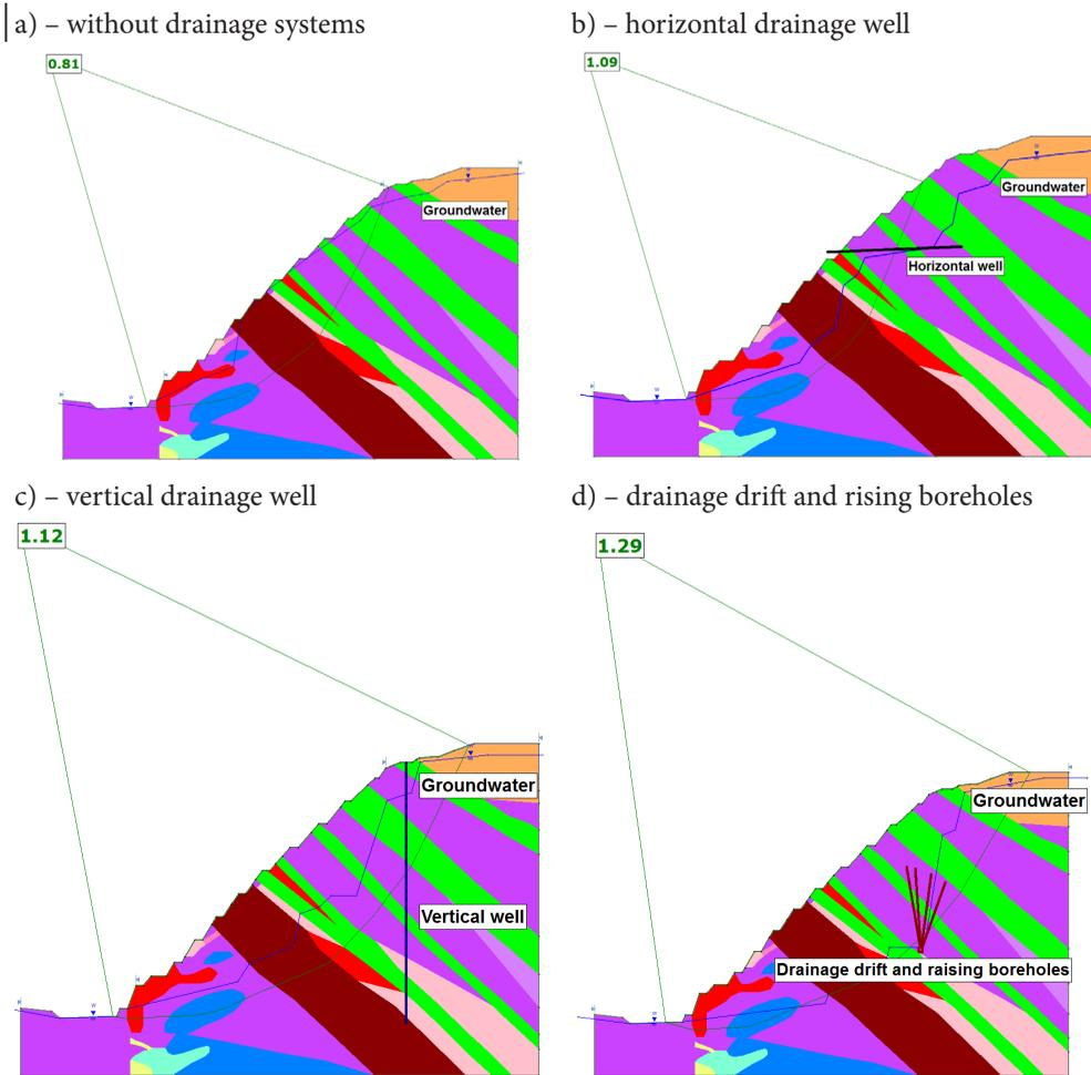
Figure 3 Safety factors of South and South-East walls using different drainage systems
