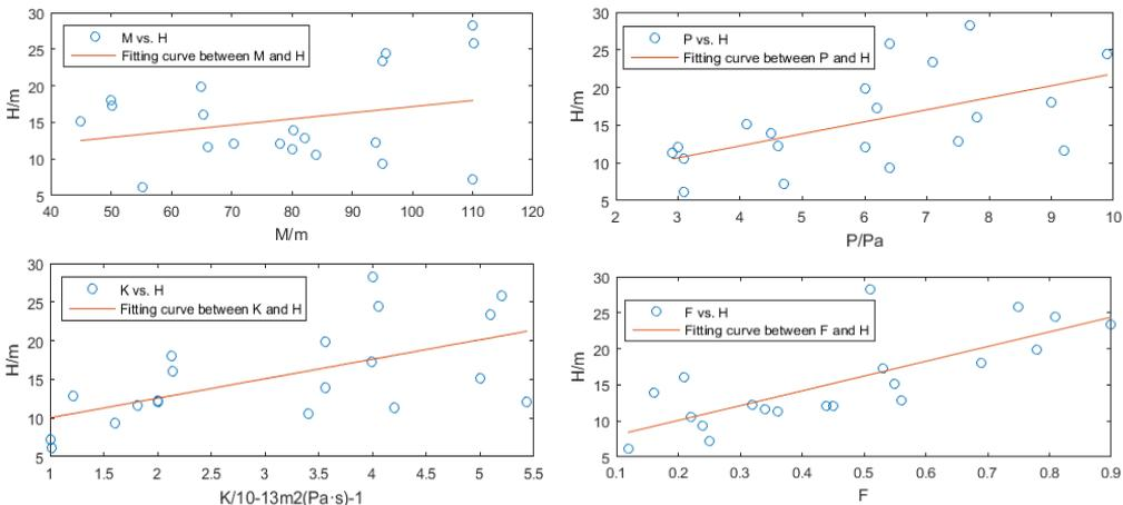
Figure 3 Fitting curve between the confined water rising zone and each influence index
