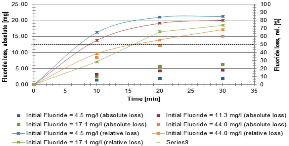
Figure 5 Absolute (abs.) and relative (rel.) Fluoride removal at different initial fluoride concentrations with ongoing treatment time.
