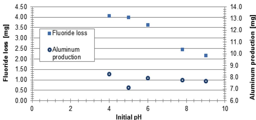
Figure 4 Fluoride removal and aluminium production at different initial pH values
