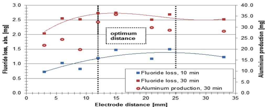
Figure 2 Fluoride removal and aluminium production at different electrode distances
