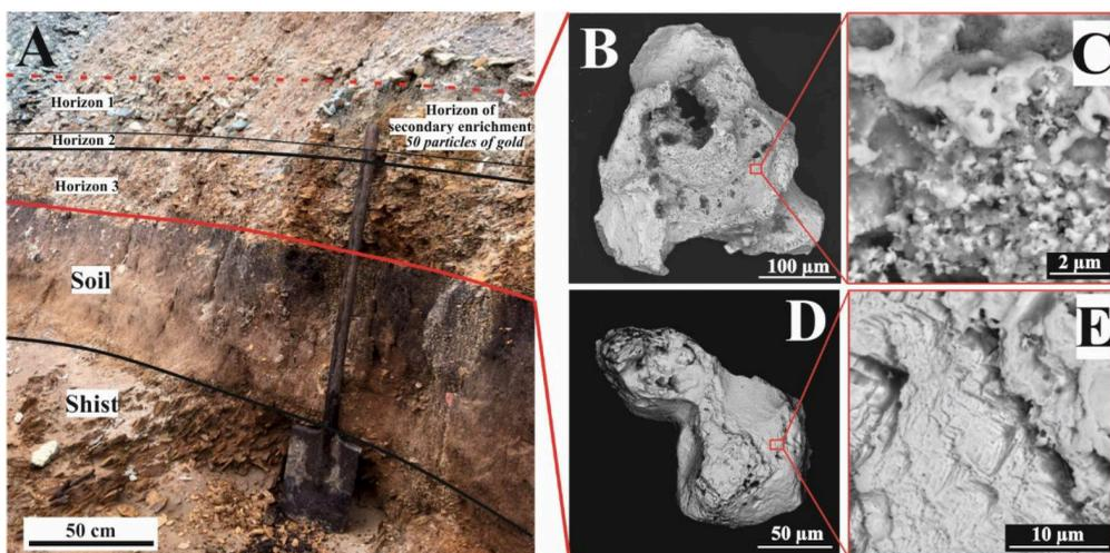
Figure 1 The Novo-Ursk deposit: A – structure of dump; B – sponge gold of crystalline form; C – increased fragment B; D – the step structure of growth gold; E – increased fragment D
