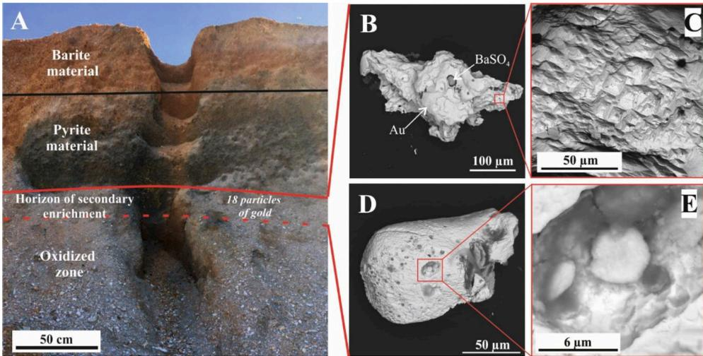
*Figure 2 The Belokluch deposit: A – structure of dump; B – crystalline form of gold with the step structure; C – increased fragment B; D – gold particle with a porous surface; E – increased fragment D newly formed phases*
