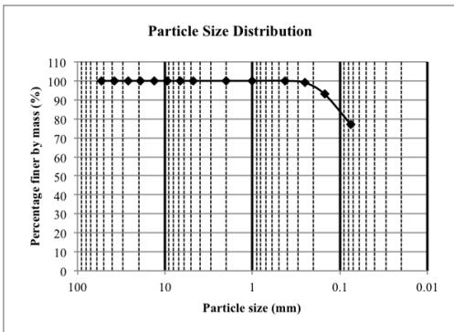
Figure 1 Particle size distribution of CFA.
