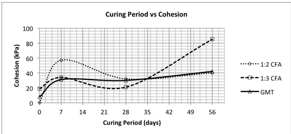
Figure 4 Relationship between curing period and cohesion.
