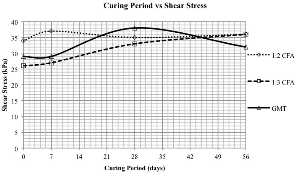
Figure 3 Relationship between curing period and shear stress.
