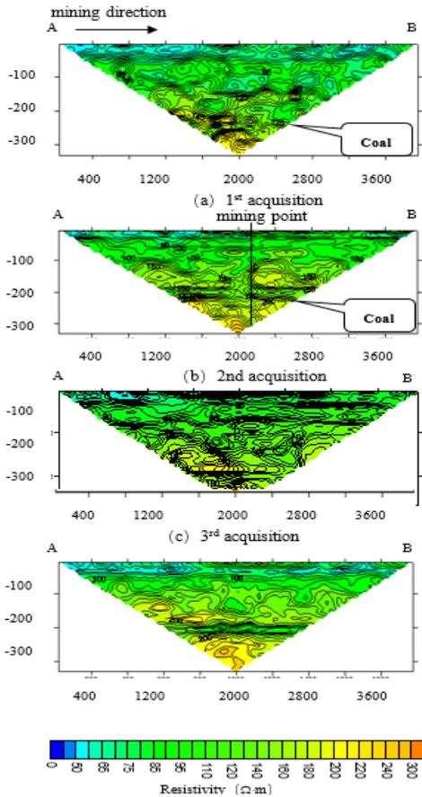
Figure 2 Geoelectrical I profiles comparison
