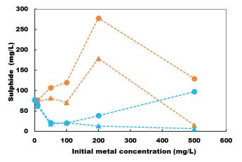
*Figure 2* Remaining sulphide ( $\Delta$ ) and total sulphide (o) production (=remaining sulphide + sulphide in metal sulphide precipitates) in the experiments carried out with SRB biomass with Co addition (blue) and Ni addition (orange).
