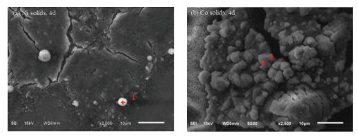
Figure 1 Secondary electron images and EDS of Ni and Co precipitates formed with biogenic sulphide.
