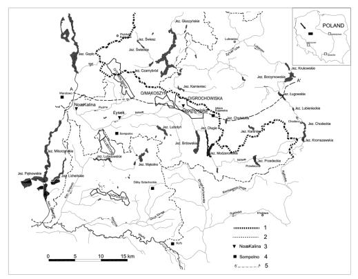
**Figure 1** Hydrographic map of the "Mąkoszyn – Grochowiska" lignite deposit area (modified from Stachy ed., 1987). Explanations: 1- first order watershed, 2-other watersheds, 3-hydrometric station, 4-precipitation station, 5-hydrogeological
