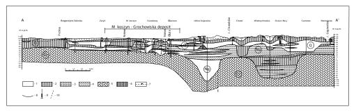
*Figure 2* Hydrogeological cross-section (Szczepinski Straburzyńska-Janiszewska, 2011). Explanations: 1-fine sands, 2-glacial tills, 3-silts, 4-clays, 5-marls and dolomites, 6-lignite, 7-Neogene-Paleogene-Mesosoic aquifer piezometric surface, 8-stratigraphic boundary, 9-screeded intervals, 10-faults.
