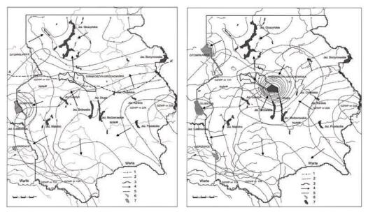
**Figure 4** Map of of hydroizohipses of the Neogene-Paleogene-Mesozoic aquifer a) in quasi-natural conditions, 2008 y, b) in hydrodynamic conditions for 2044 y, computer model prediction. Explanation: 1-piezometric surface of Neogene-Paleogene-Mesosoic aquifer, 2-range of the cone of depression, 3-model boundary, 4-groundwater flow direction, 5-hydrogeological cross-section, 6-mine drainage area, 6-pit lakes
