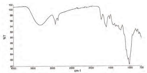
Figure 3 FT-IR results of the orange peels powder.
