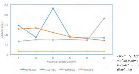
Figure 5 Effect of various volume of antiscalant on CaCO3
