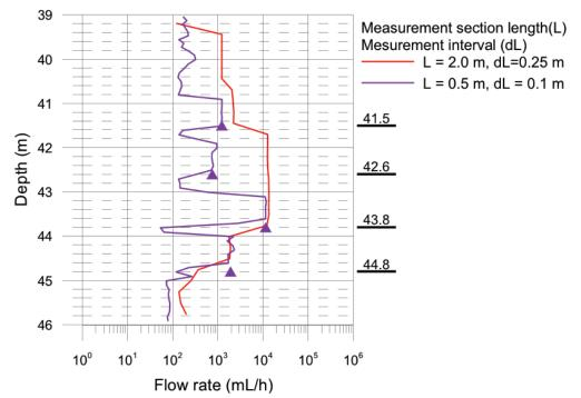
Figure 3. Fracture flows measured with 0.5 m and 2 m measurement section lengths.
