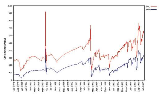
*Figure 1* Concentration of sulphates and total dissolved solids from September 1978 to July 2007 in the Middelburg Dam (Source: Department of Water Affairs)
