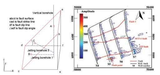
Fig.6 Fault detection based on radial jetting
