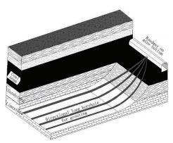
Fig.3 Schematic of underground directional boreholes
