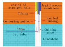
Fig.2 Schematic radial jet process
