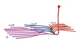
Fig.1 Subarea layout of directional boreholes
