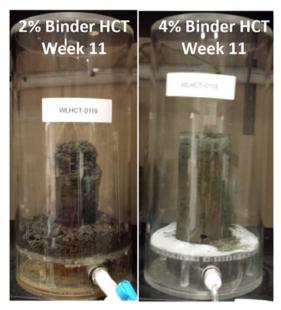
**Figure 3** Photos of 2% (left) and 4% (right) HCTs of cemented paste tailings cylinders at 11 weeks of testing.
