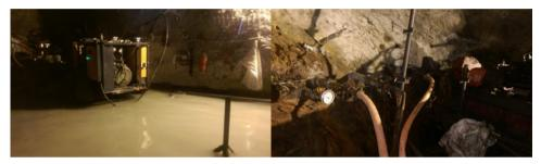
**Figures 2 & 3.** Left: Test terminated early as water levels reached the pre-arranged shut-in trigger level. Right: Example drain holes with manual read pressure gauges and 2 open holes with hoses attached for barrel-fill flow rate tests.
