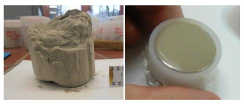
Figure 3 left: drill core sample; right: cup with dried, homogenized tailing material
