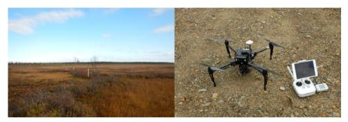
**Figure 3** Viiankiaapa mire (on the left) and the UAV-TIR platform (Matrice 100) with TIR and RGB cameras (on the right).
