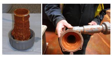
**Figure 3** Blocked strainer filter on mine water feed to heat exchanger (left) and ochreous deposits on the heat exchanger inlet (right).
