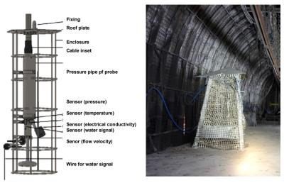
Figure 5: Underground probe for long term observation in closed mines.
