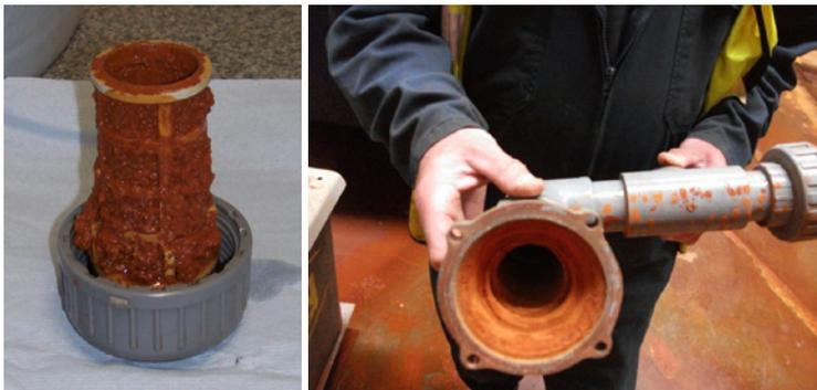
**Figure 3** Blocked strainer filter on mine water feed to heat exchanger (left) and ochreous deposits on the heat exchanger inlet (right).
