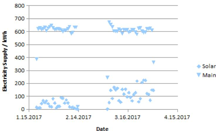
**Figure 4** Solar (blue diamonds) and main (red squares) daily electricity supply at Dawdon MWTS during early 2017 follow installation of main supply meter telemetry. See text for further explanation.
