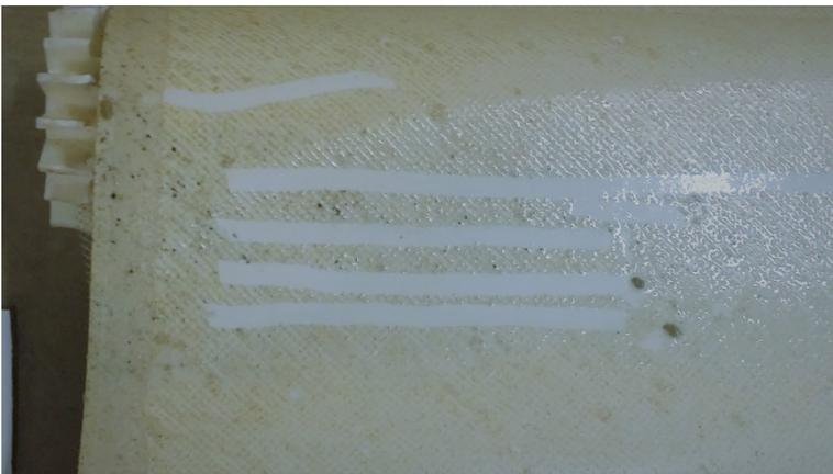
**Figure 1.** Biofilm on the RO membrane. White marks represent sampling areas where biofilm was scratched, revealing the membrane.
