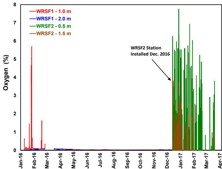
**Figure 3** Oxygen concentration within the WRSF sealing layer.
