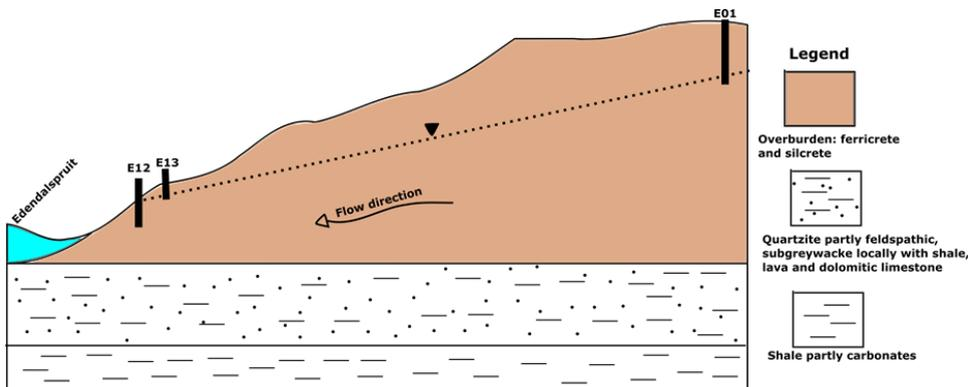
**Figure 2** Conceptual model of hydrogeology of the abandoned Edendale Lead Mine
