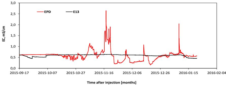
**Figure 4** EC measurement in shaft E13 and the discharge point of the abandoned Edendale Lead Mine during the tracer test
