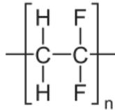
**Figure 1** Molecular Structure of Polyvinylidene Fluoride
