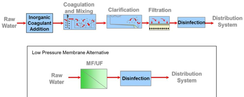
Figure 4 Membrane versus conventional process treatment
