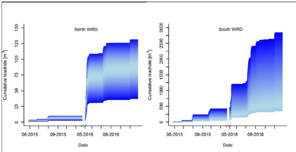
**Figure 4** Cumulative leachate generation from north and south waste rock dumps. Color-coding is based on rating curves where lighter blue indicates the lowest absolute sum of residuals, i.e. the best fit to data.
