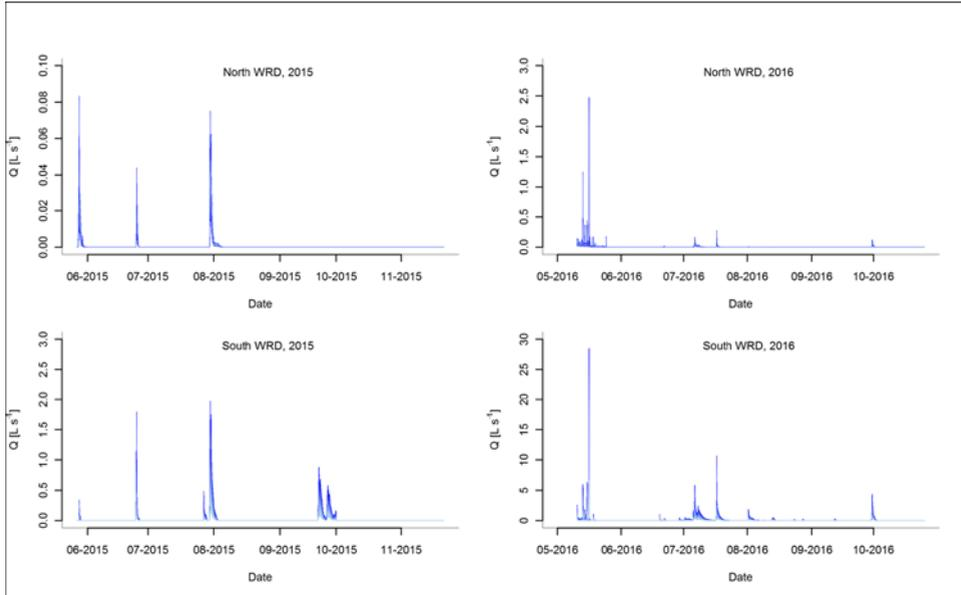
**Figure 3** Leachate discharge from north and south waste rock dumps, calculated from rating curves and measured water levels. Note that discharge scales are different for each diagram.
