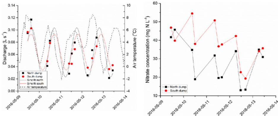
**Figure 5** Left: Leachate discharge from north and south rock dump during snowmelt in 2016. Leachate discharge has been fitted with a sine curve to illustrate the cyclicity in discharge, relative to air temperature (right axis). Right: nitrate concentrations during snowmelt.
