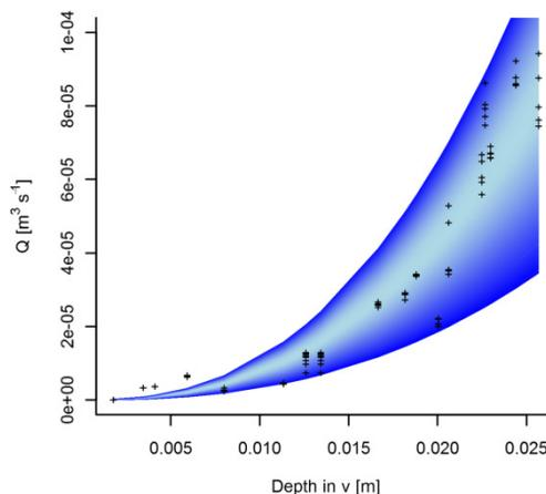
**Figure 2** Rating curve for discharge from the north waste rock dump. Lighter blue indicates the lowest absolute sum of residuals, i.e. the best fit to data, while the darker blue is a poorer fit.
