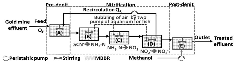
**Figure 1** Pilot-scale system with continuous flow
