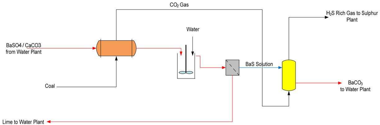
**Figure 4** The chemical recovery process
