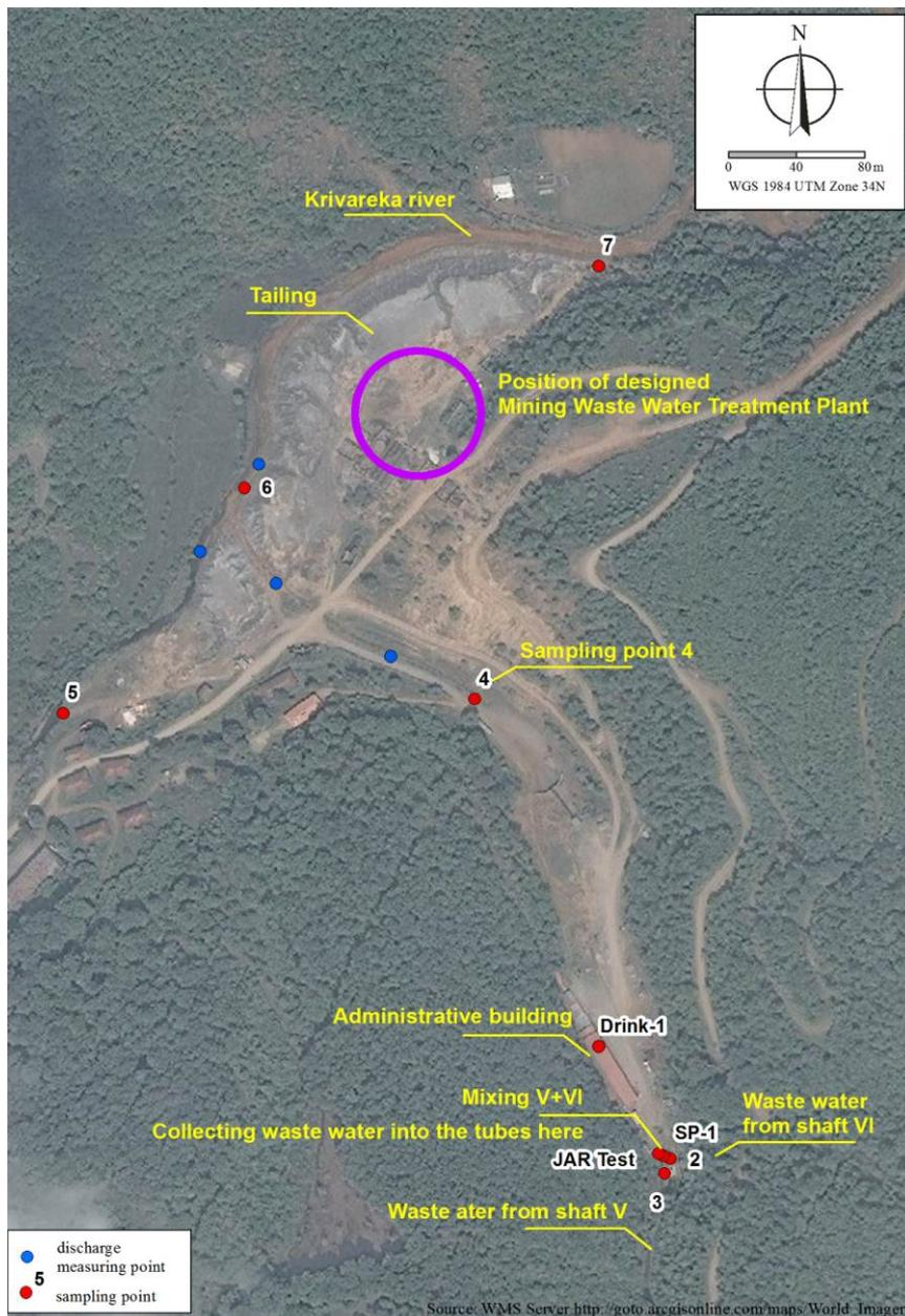
**Figure 4** Sampling and flow measurement locations
