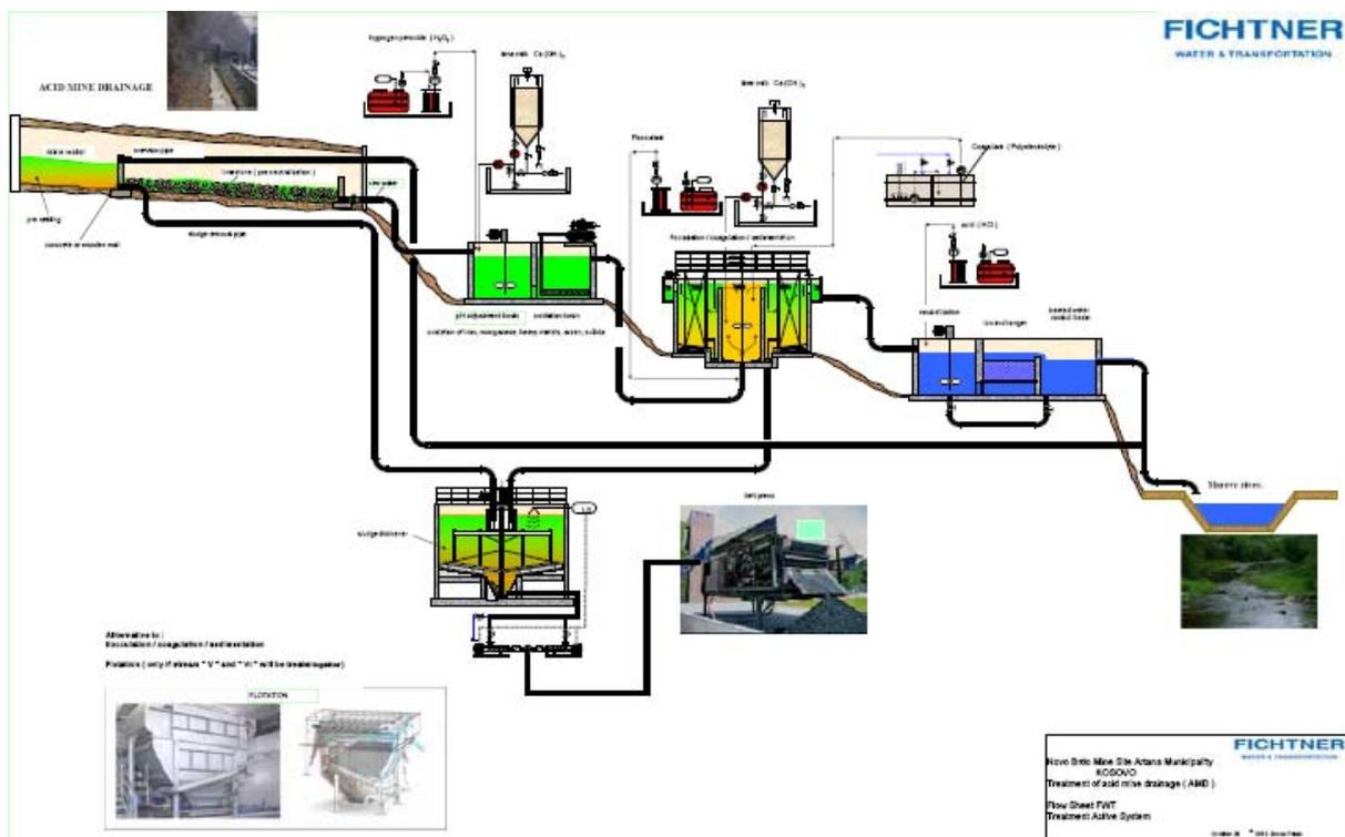
Figure 7 Technical design of an Active Treatment Plant
