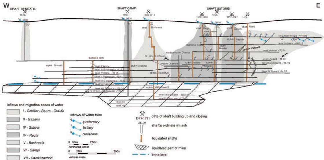
Fig. 3 Scheme of the groundwater inflow zones to the "Bochnia" salt mine
