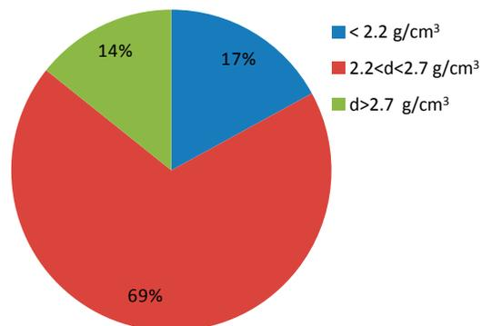
**Fig. 1** Mass department of coal discards to density fractions.
