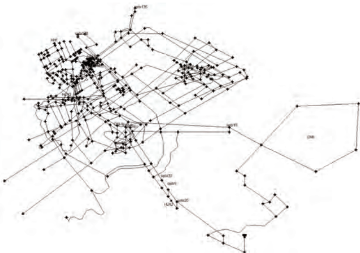
Figure 3 Complex mine geometry with main connections used for the modeling of flow and heat by the adapted EPANET-code.
