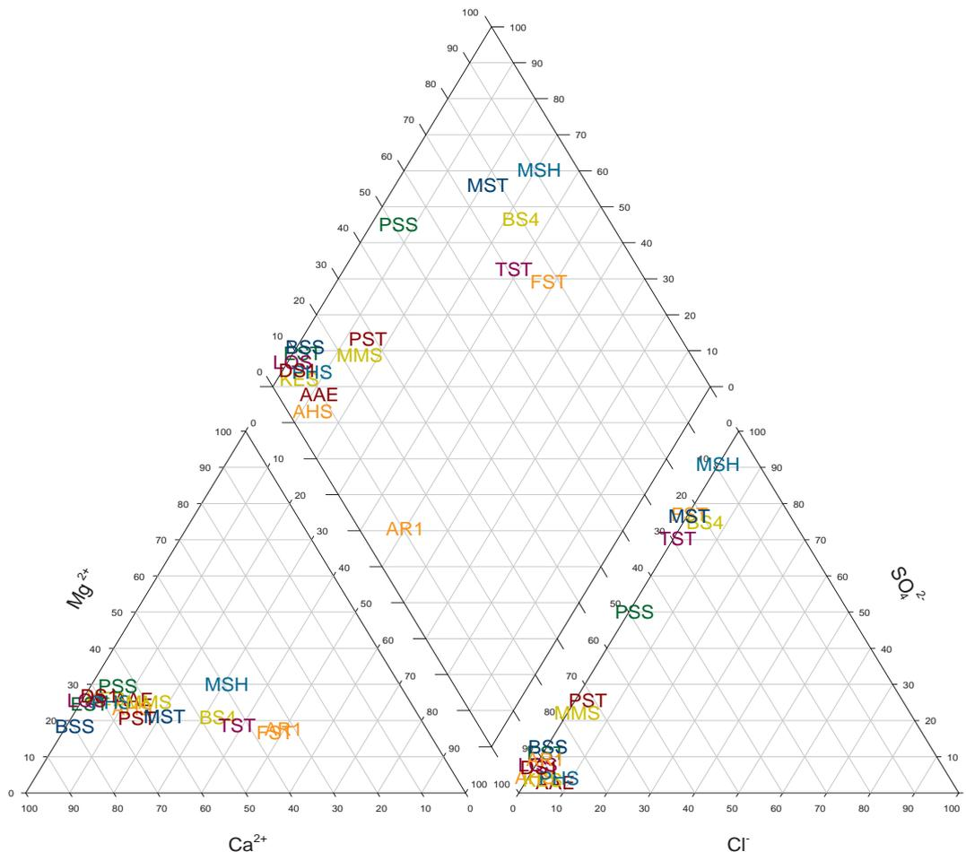
Figure 2. PIPER (PIPER 1944, 1953) diagram of the 17 mine water discharges in the Southern Bavarian pitch coal mining district. The labels are meant as an indication for the total water chemistry, not the chemistry of the single samples.
