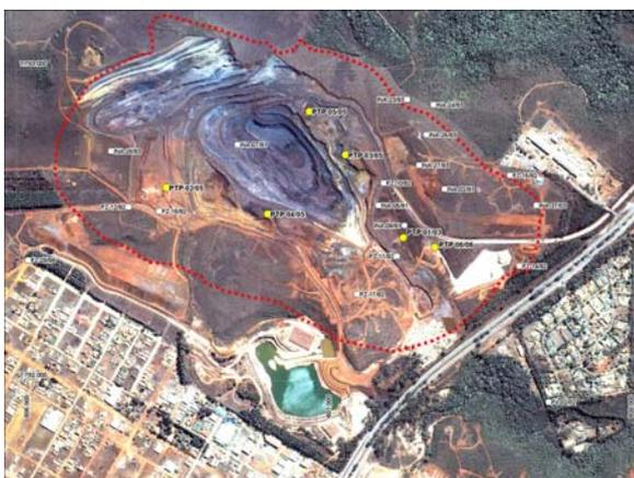
Figure 5. Location of the dewatering wells and piezometers in the close neighbourhood
