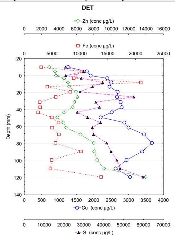
Figure 7 Dept Profiles obtained by the porewater peeper sampler
