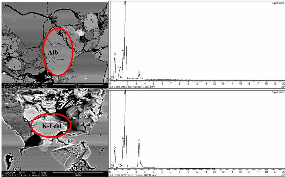
Figure 7. SEM photographs of sandstone samples showing plagioclase feldspar (albite) and K-feldspar from Brandspruit and Vaalkrantz Colliery
