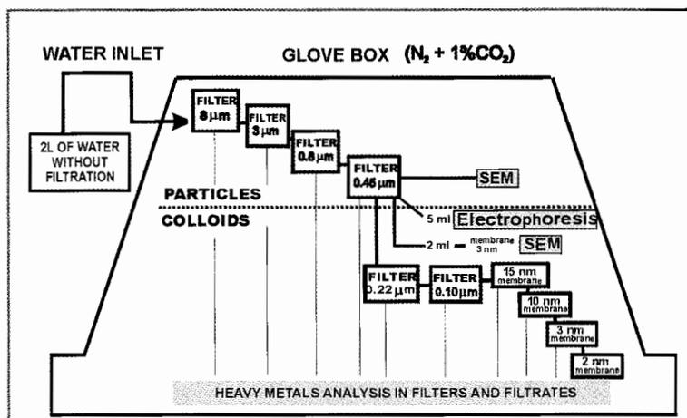
Figure 1. Suspended particles and colloids fractionation system in a glove box to characterise the association of heavy metals in the waters affected by the spill of Aznalcóllar mine.
