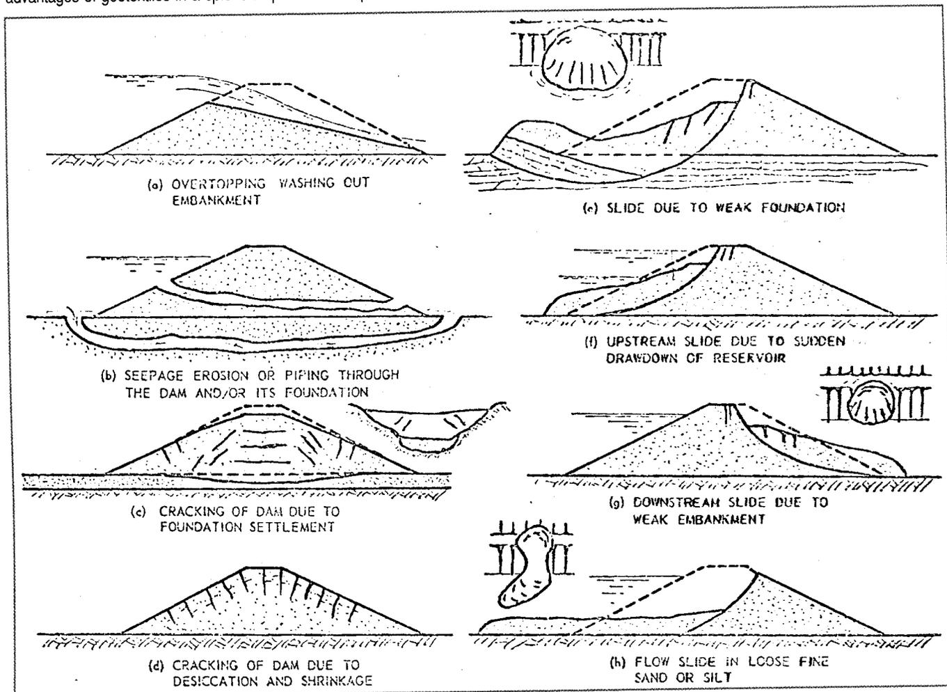
Figure 1. Failure of Earth Dams.
