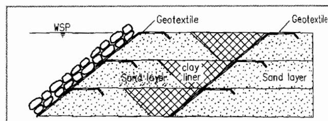
Figure 8. Installation of geotextiles as filter in the dam (hydraulic fill dams).
