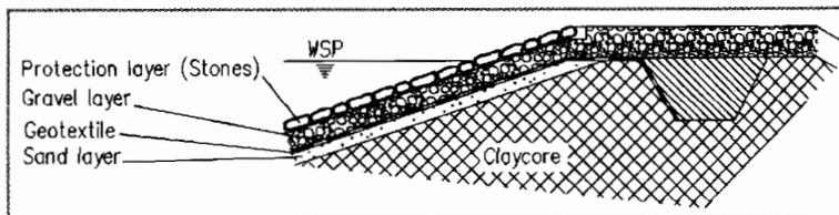
Figure 4. Geotextile on the upstream face as separation layer and filter.
