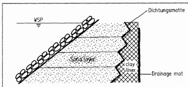
Figure 11. Installation of sealing mats.
