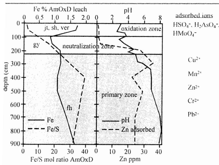
Figure 1. Typical tailings stratigraphy (e.g. Pluques A2) with secondary mineralogy (jarosite = jt, schwertmannite = sh, vermiculite-type mixed layer clay mineral = ver, gypsum = gy, ferrihydrite = fh), pH, and Fe, and Fe/S mol ratio variation in the ferric oxyhydroxide leach ( $\text{NH}_4\text{-OxD}$ ). Adsorbed Zn is from a 1M  $\text{NH}_4$ -Acetate leach). The general trend of adsorbed ion species is shown at the right.
